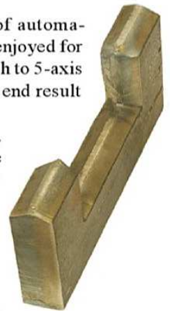
A test part with a symmetrical K bevel cut in three passes on 25.4mm plate, 10, 5.4, 10 at 30 degrees.
