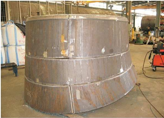
Variable dihedral K preparations generated by FastCAM.
